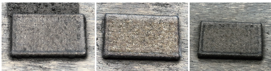
图4 扫描速度为8mm/s、10mm/s时的熔覆样件表面 Fig.4 Surface of the cladding samples when the scanning speed is 8mm/s, 10mm/s
