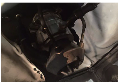
图2 被挥发的Ti污染的激光熔覆沉积系统 Fig.2 Laser cladding deposition system polluted by volatile Ti
