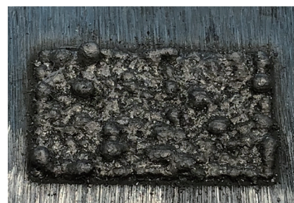
图3 扫描速度为12mm/s的熔覆样件表面 Fig.3 Surface of the cladding sample when the scanning speed is 12mm/s
